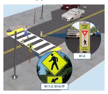
Warning sign types for midblock crosswalks and trail crossings shall be installed as follows:
