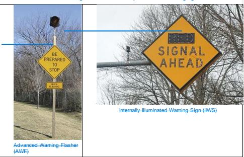
AWF or HWS should only be installed in response to a specifically correctable problem, not in anticipation of a future problem. Generally, AWF or HWS implementation is appropriate only at high speed locations. Before an AWF or HWS is installed, other remedial action should be considered.
